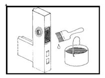
If any part of a previously treated external door or door frame is cut or drilled, swab the newly exposed timber with a suitable organic solvent preservative treatment and re-coat with primer or stain.
